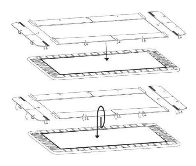
On the bottom side of the pad there are eyelets to connect the pad to the frame. Pull the elastic bungee(7) through the eyelets and tie it around the frame.
