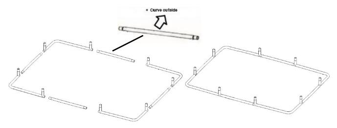
STEP 2: Assemble the top frame in the same way as the bottom frame (see step 1)
