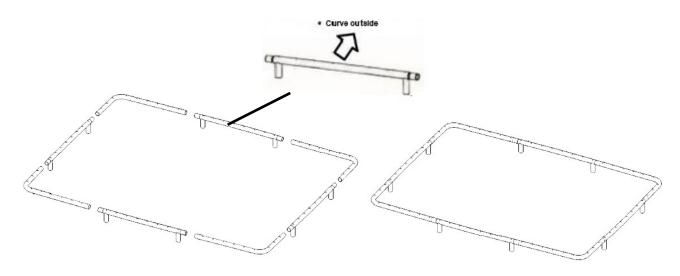
STEP 3: Now place the top frame on the bottom frame and let all parts rest on the "spring buttons". When all parts rest on the "spring buttons" you can press them and then slide the top frame over the bottom frame from above.
