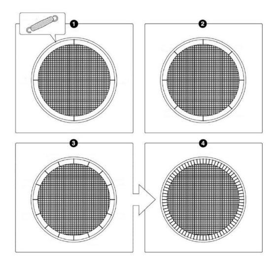
STEP 5: Place the pad(6) on the frame so the springs and frame are completely covered. Also make sure the safety instructions are on the entrance side of the trampoline.
