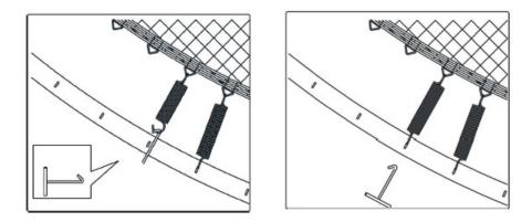
The springs should be evenly distributed over the mat, see the image below how to divide the springs
